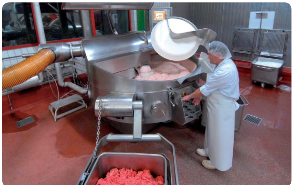
In the machine referred to as the cutter, the meat is seasoned and prepared as sausages meat.
