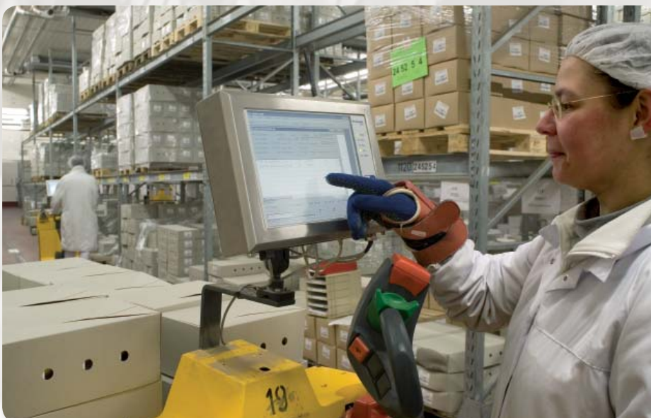
An order picker retrieves data using the noax IPC. She is wearing a scanner on her right wrist.
